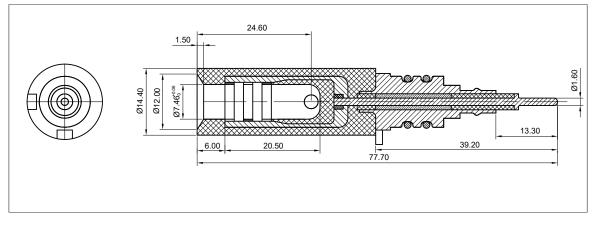
www.sunkye.com D011 High Temperature & High Pressure Conne
